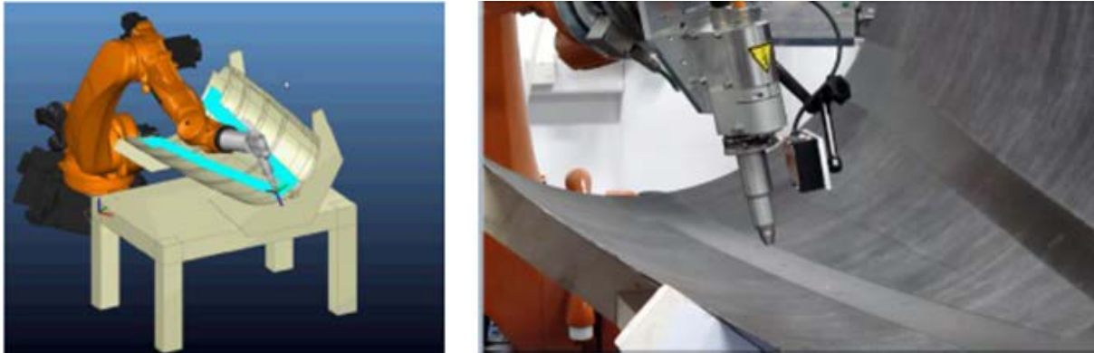
Figure 5: Automatic plasma treatment prior to bonding
